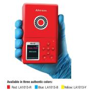
Palm PCR™ - LA1013 is an extended version of the Palm PCR™ series. Further to the full capacity of performing PCR reactions, multistep isothermal functions are provided. The LA1013 model represents a complete solution for performing both PCR reactions and related biochemical processes such as reverse transcription and DNA preparation, in a single instrument.
