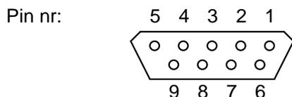
Fig.3. Remote control socket seen from outside.
