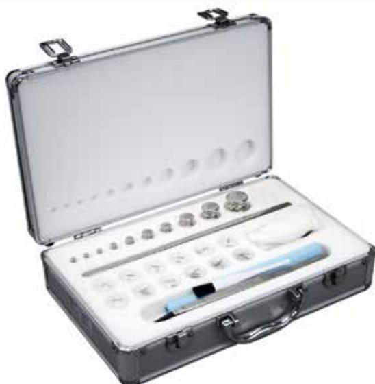
OIML weight sets include a complete group of test weights that can meet requirements for testing to OIML standards. E2 weight sets provide a high level of accuracy and are ideal for calibrating analytical and precision balances. M1 weight sets offer a lower level of accuracy, but are affordable and ideal for calibrating compact portable balances and bench scales.
